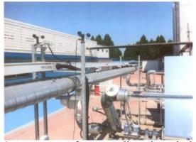
Anemometer for recording the wind around collectors.
