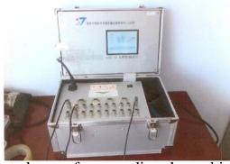
Data logger for recording the ambient temperature, radiation and wind speed
