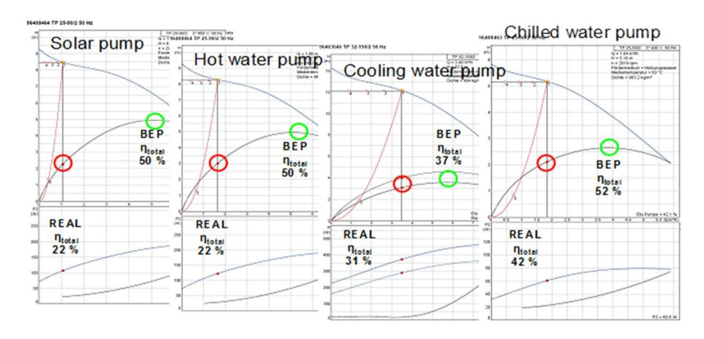
⇒ Nominal operation point has to be designed slightly right the BEP in order to achieve good system performance in part load
