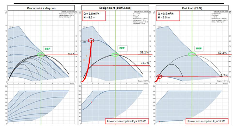
⇒ Worse pump efficiency despite high efficiency pumps
