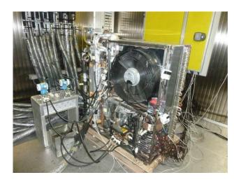
The thermodynamic cycle is a dual lift water ammonia low temperature driven absorption cycle, in which the refrigerant flow self-adapts to the evaporator and absorber loads, making the system capable of adapting to variable loads and boundary conditions.
