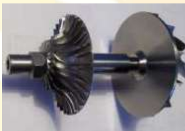
Turbo Expander/Compressor AC-Sun, Denmark in TASK 38
