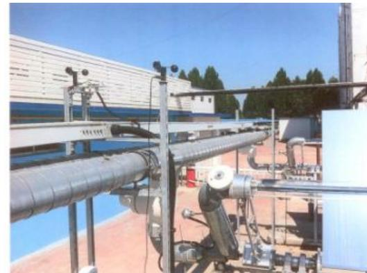
Anemometer for recording the wind around collectors.
