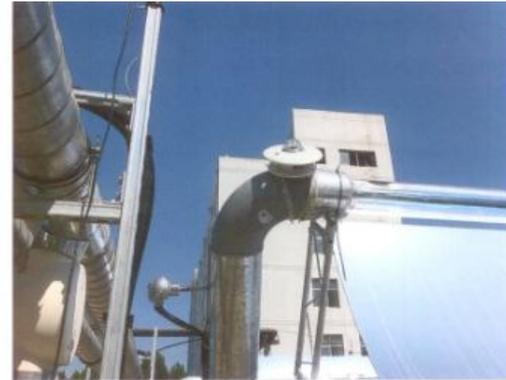
Pyranometer for recording the solar radiation
