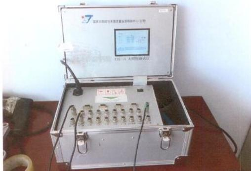
Data logger for recording the ambient temperature, radiation and wind speed
