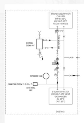
Absorption Chiller: Heat input 500kW Single Stage Machine 95 C f, 85 C r
