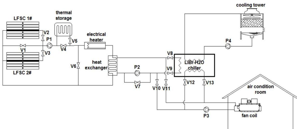
Figure 23: Schematic of the solar energy and heat storage system (Source: SJTU)
