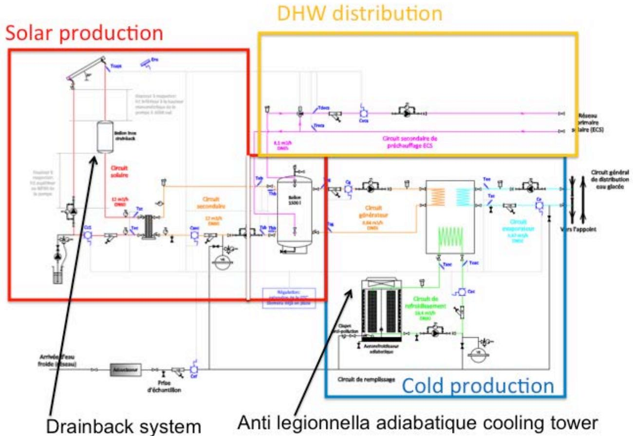
Figure 7: Detailed hydraulic scheme of the SHC system of the two buildings (Source: TECSOL)
