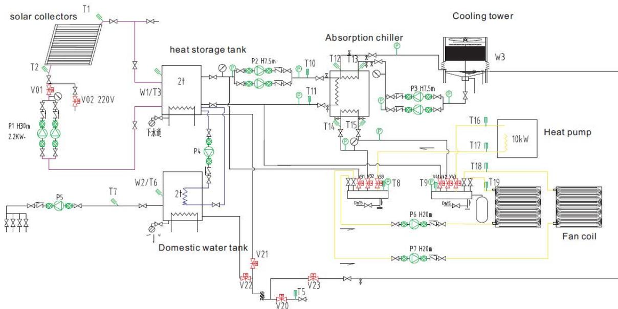
Figure 19: Scheme of the solar cooling system at the Linuo office building (Source: SJTU)
