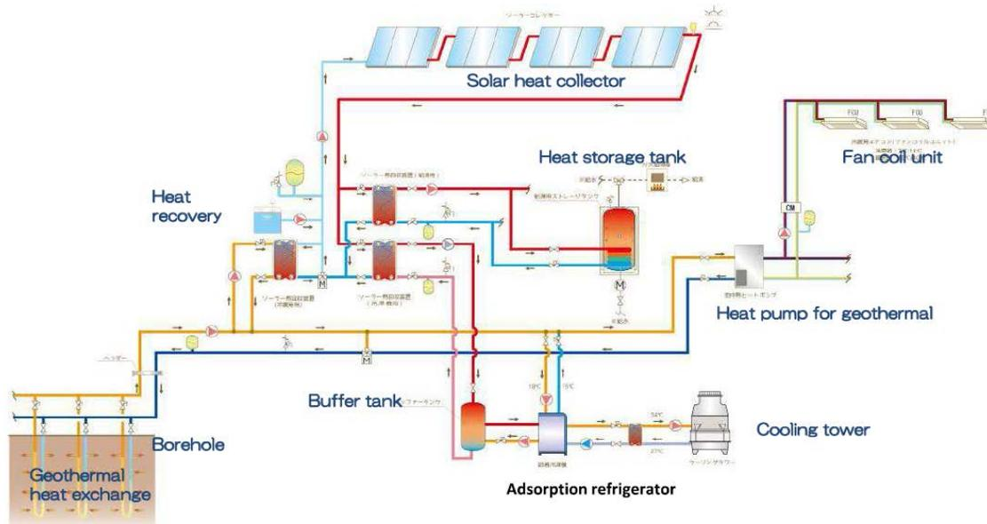
**Figure 29: System flow of the cooling system (Source: Osaka Technocrat Ltd.)**
