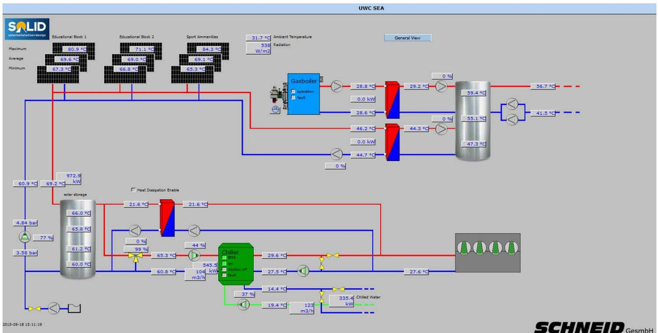
Figure 17: Monitoring scheme of the solar cooling system at the UWC (Source: SOLID)
