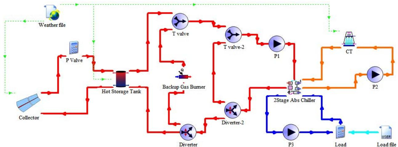
**Figure 30: TRNSYS schematic of simulated solar cooling system with double-effect absorption chiller (Source: CSIRO)**
