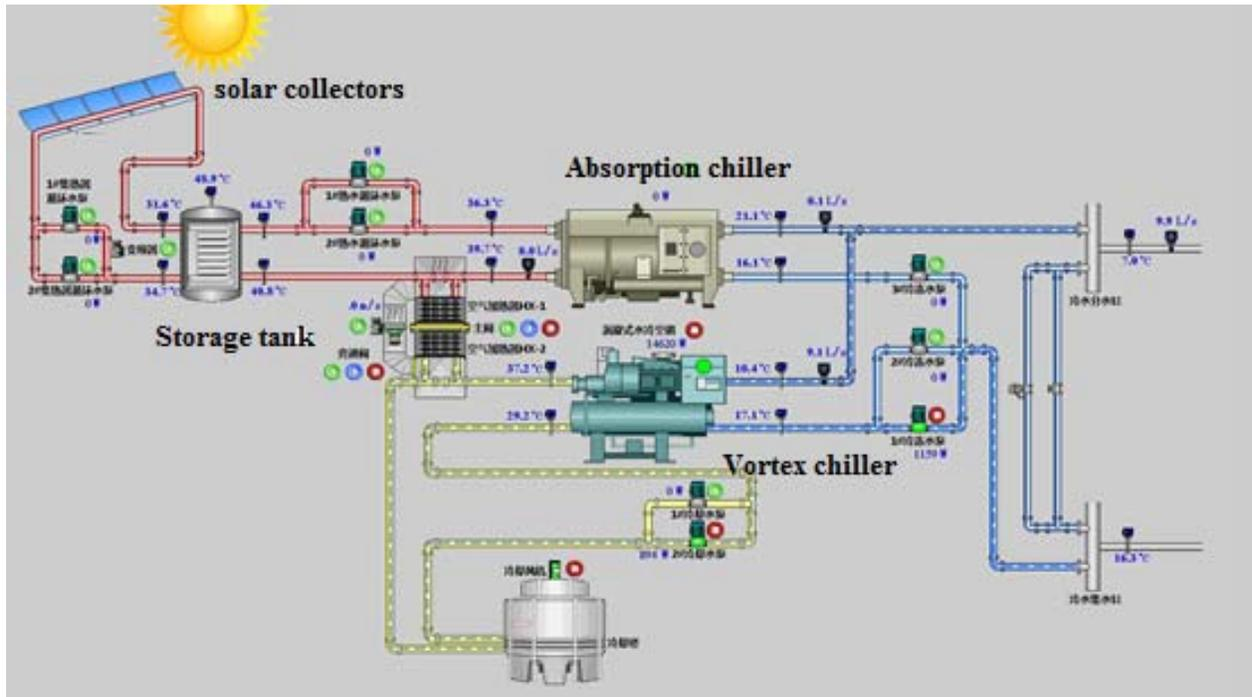
Figure 21: Scheme of the absorption chiller system with the vortex chiller (Source: SJTU)
