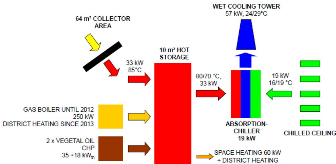
Figure 12: Scheme of the solar cooling system at Feisfritzwerke (Source: UIBK)
