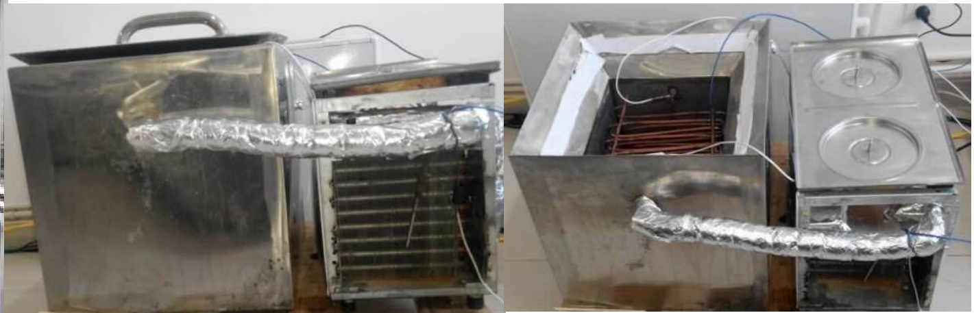
Photos of ice storage air conditioning
