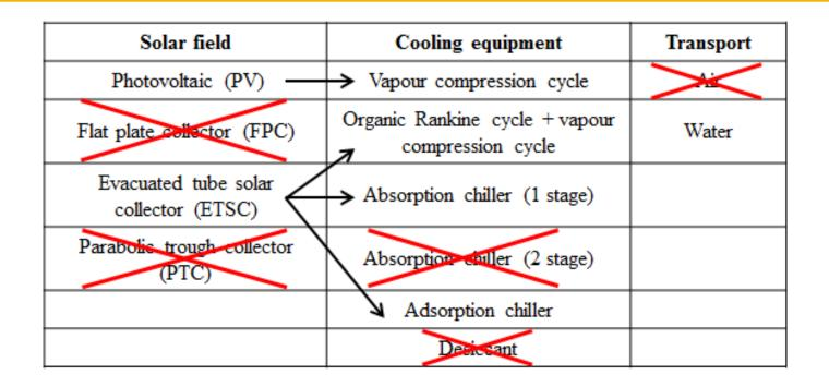
System overall efficiencies PV panel  $(0.15) + VCC (4) = \sim 0.6$ ETSC  $(0.5) + ORC (0.1) + VCC (4) = \sim 0.2$ ETSC (0.5) +one-stage absorption chiller  $(0.7) = \sim 0.35$ ETSC (0.5) +adsorption chiller  $(0.7) = \sim 0.35$
